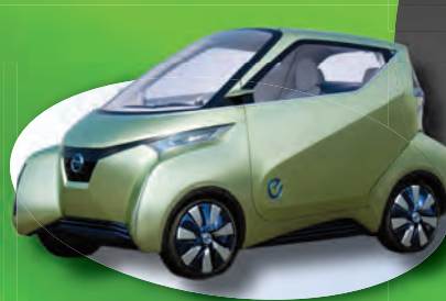
Nissan Pivo 3: EV commuter car has motors in the wheels to allow maximum interior room and lets each wheel rotate so this three-seater can move sideways into tiny parallel parking spaces.
