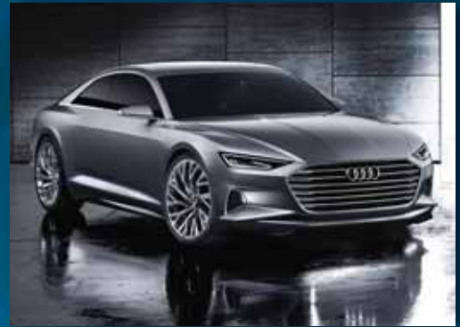
Audi Prologue: Audi's pillar-less coupe has a 605-hp twin-turbo V8 and "rear-wheel steering," which allows the rear wheels to be angled up to five degrees for better high-speed handling.
