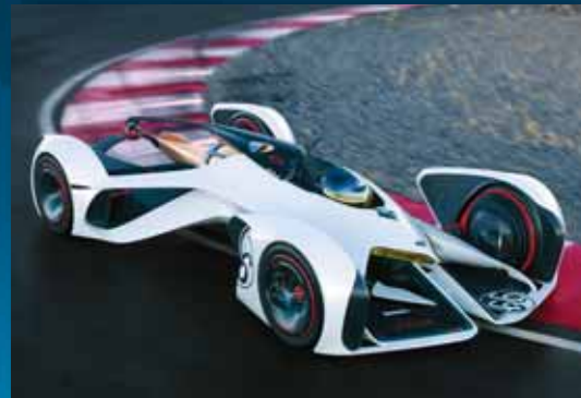
Chevy Chaparral 2X Vision Gran Turismo: In this laser-powered virtual car, the “driver”—who lies face down with legs splayed—wears a helmet, and instruments are projected onto the visor.
